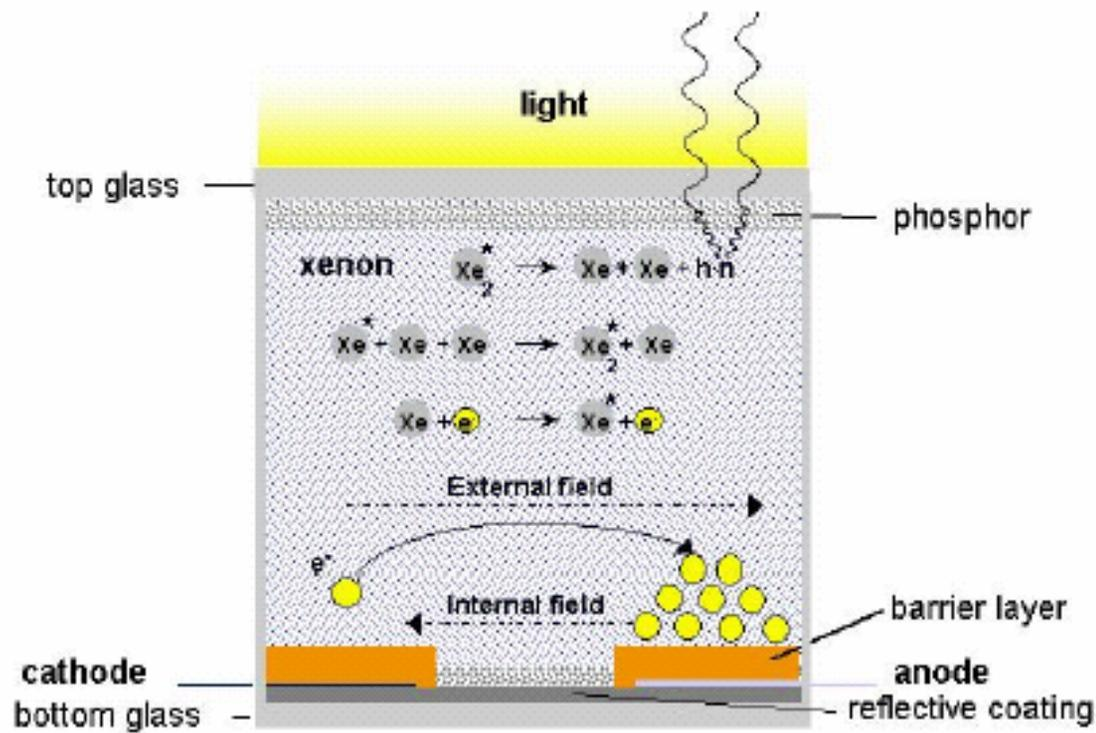
Figure 1 : Schematic view of the xenon barrier discharge
