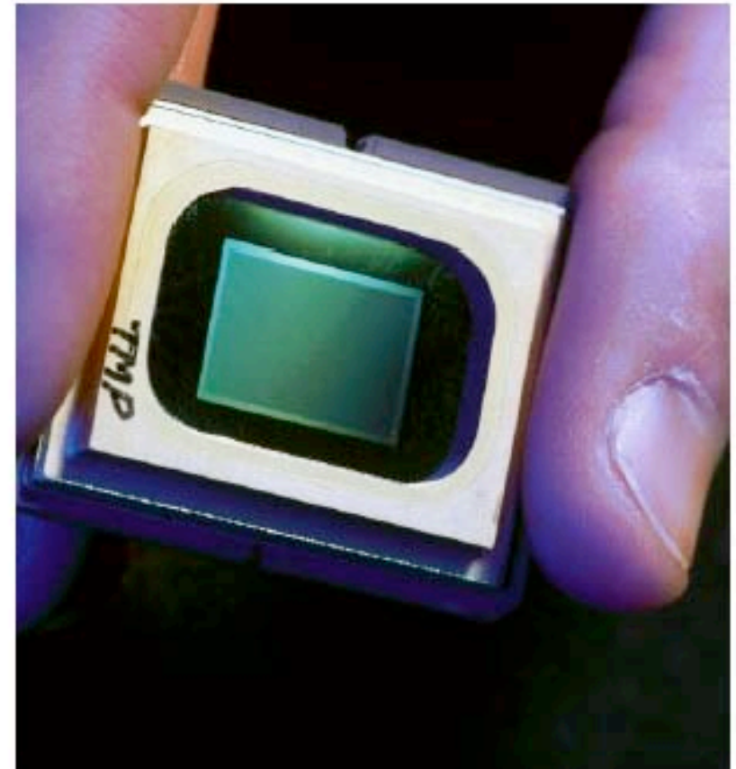
Picture 3: TI DMD Chip with 800 x 600 mirrors 16 \mu m x 16 \mu m
